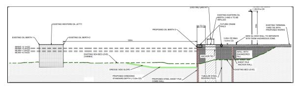
Figure 5-4: Cross Section G-G Proposed Oil Berth 03 and Infilling of Oil Berth 04 Basin Source: Drawing no CP1770-BLP-03-ZZ -M2-MA-0301 prepared by Atkins Byrne Looby Consulting Engineers
