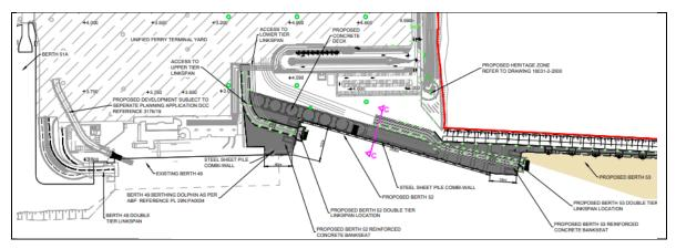
Figure 5-2: Plan view of Modified Berth 52
