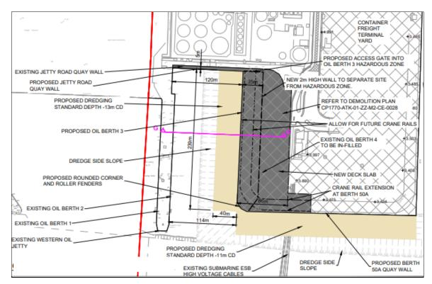
Figure 5-3: Plan View of Proposed Extension to Berth 50A, Redesigned Oil Berth 03 and Infilling of Oil Berth 04 Basin
