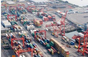
*Secondary handling equipment* refers to the equipment (usually gantry cranes of one type or another) used to store containers in back areas in large stacks.
