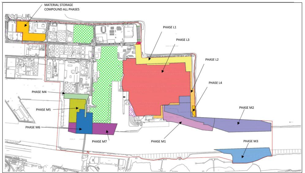
Figure 3-14 Plan of general project phasing
