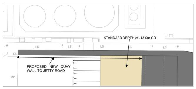
Figure 3-7 Plan of proposed Jetty Road Quay Wall
