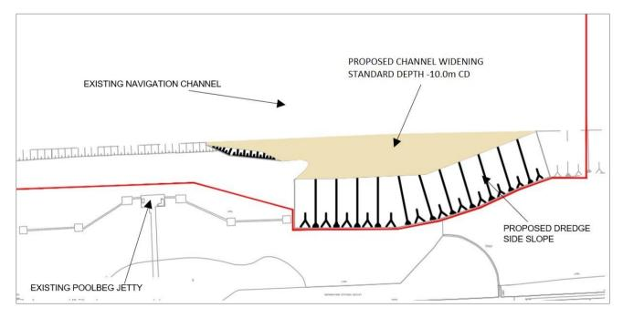
Figure 3-8 Plan view of proposed channel widening works
