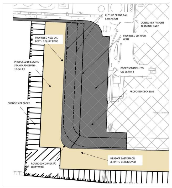
Figure 3-6 Plan view of proposed Oil Berth 3
