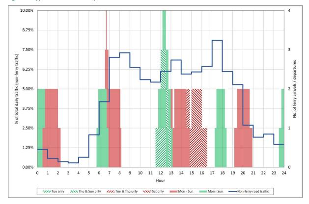
Figure 1: Typical 24-hour traffic profile in Dublin Port
