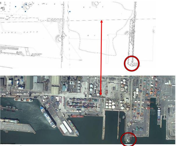
Figure 3 19<sup>th</sup> century OS map extract compared with modern satellite image showing location of pier head terminus and modern infill to facilitate the port infrastructure.
